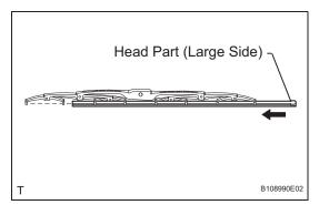
(c) Attach the head part (large side) of the wiper rubber to the rear end side claw of the wiper blade.
