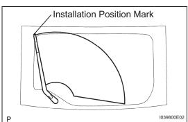
(d) Install the arm and blade with the nut. Make sure that the arm and blade comes to the position shown in the illustration.
