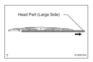
(b) Remove the wiper rubber in the direction indicated by the arrow in the illustration.
