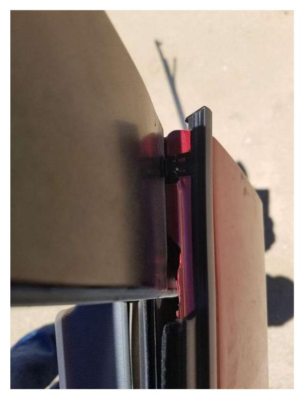
Just carefully take that clip out. Reverse install is literally a 'snap'. Do not use any metal objects as you may scratch you car's finish; I used no tools at all...
