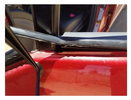
Once that groove is loosened, continue slowly to ward the back of the door until it is all loose (pic4).
