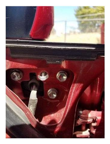
Then I carefully bent the strip inward toward the cabin to release the groove that spans the entire way back. You can see the groove on the bottom of the stripping in (pic3) even though that is a pic from the outside of the car.
