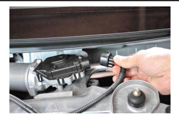
4.) Disconnect the main wiper motor harness. Remove four plastic fasteners by pinching the tabs underneath with needle nose pliers and set the wiring loom aside. [Fig. 3]
