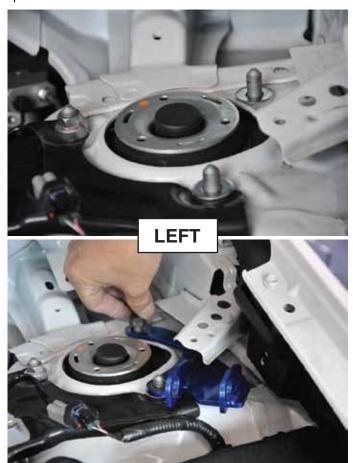
7.) Install the main bar with the washers and crush washer in this order. Hand tighten both ends, then torque down with a 17mm wrench and hex allen head driver.
