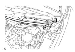
(1) Engage the 2 claws and 3 guides to install the center cowl top ventilator cover.
