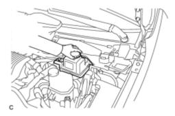
(2) Add brake fluid into the reservoir between MAX and MIN level on the brake fluid reservoir.
