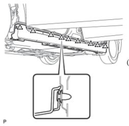
(b) Engage the 9 clips to install the body rocker panel moulding assembly.
