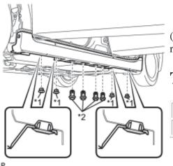
(f) Remove the 4 side mudguard retainers and 4 No. 2 side mudguard retainers.
