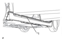
(a) Put protective tape around the body rocker panel moulding assembly.
