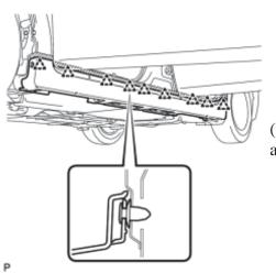
(g) Disengage the 9 clips to remove the body rocker panel moulding assembly.
