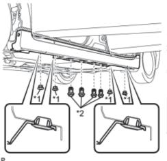
(c) Install the 4 No. 2 side mudguard retainers and 4 side mudguard retainers.
