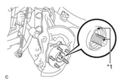
(a) Put matchmarks on the front drive shaft assembly and front axle hub sub-assembly.
