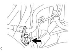
(a) Remove the bolt and separate the front flexible hose from the steering knuckle.
