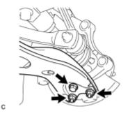
(a) Install the front No. 1 lower suspension arm sub-assembly to the front lower ball joint with the bolt and 2 nuts.
