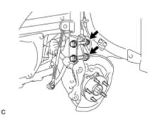
(a) Install the front axle assembly to the front shock absorber with the 2 bolts and 2 nuts.
