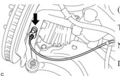
(b) Install the front speed sensor to the steering knuckle with the bolt.
