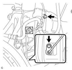
(a) Remove the 2 bolts and clamp, and separate the front speed sensor.
