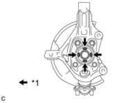
(b) Install the front axle hub sub-assembly and front disc brake dust cover with the 4 bolts.
