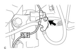
(a) Install the front speed sensor and front flexible hose to the front shock absorber with the bolt and clamp.
