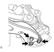
(a) Remove the bolt and 2 nuts, and separate the front No. 1 lower suspension arm sub-assembly from the front lower ball joint.
