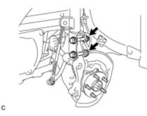
(a) Remove the 2 bolts, 2 nuts and front axle assembly.
