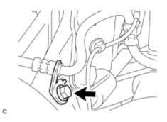
(a) Install the front flexible hose to the steering knuckle with the bolt.
