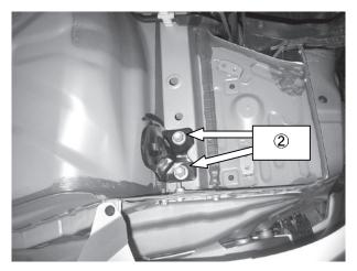
3.) Install the powerbrace under the brackets that were taken off in the previous step. Also reuse the factory bolts.
