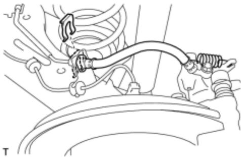
(b) Remove the clip and separate the rear flexible hose LH.
