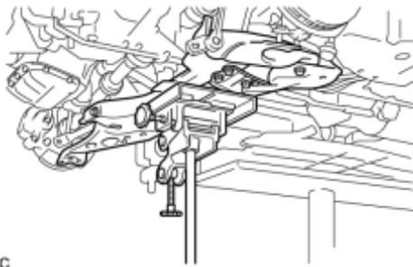
(c) Using a transmission jack, support the front suspension crossmember sub-assembly.
