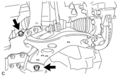
(a) Temporarily install the front No. 1 lower suspension arm LH to the front suspension crossmember with the 2 bolts and nut.
