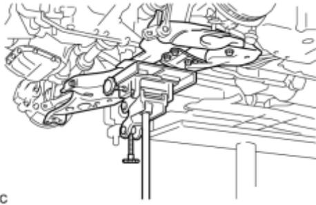
(a) Support the front suspension crossmember with a transmission jack.
