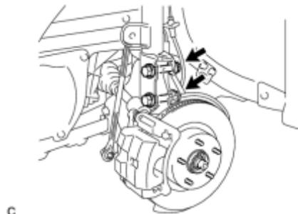
(c) Remove the 2 bolts and 2 nuts, and separate the front shock absorber with coil spring (lower side) from the steering knuckle.
