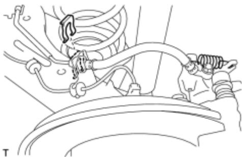
(b) Connect the rear flexible hose LH to the rear axle beam assembly with a new clip.
