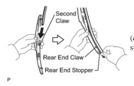
(c) After pushing the wiper rubber through the rear end claw, allow it to stick out from the rear end stopper.
