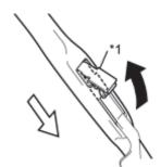
(a) Remove the holder of the front wiper blade as shown in the illustration.
