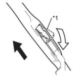
(a) Install the front wiper blade as shown in the illustration.
