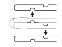
(b) Remove the 2 wiper rubber backing plates from the wiper rubber.
