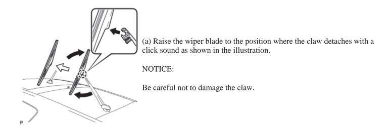
(b) Pull the wiper blade straight toward to remove it from the wiper arm.
