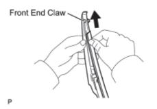
(d) Slide the wiper rubber through the front end claw.
