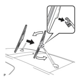
(b) Engage the claw to install the rear wiper blade as shown in the illustration.
