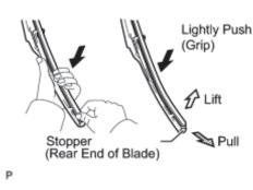
(a) Lift and pull the end of the wiper rubber protrusion from the blade stopper as shown in the illustration.
