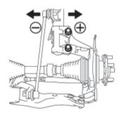
(e) Fully push or pull the front axle hub in the direction of the required adjustment. (Step B)
