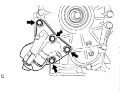
(i) Temporarily tighten the oil filter bracket with the 4 bolts.
