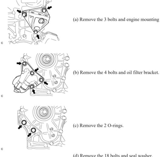
(a) Remove the 3 bolts and engine mounting bracket RH.
