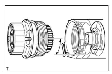
(6) Using SST, tighten the oil filter cap assembly.
