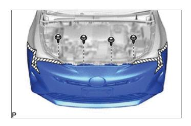
(j) Remove the 2 clips and front bumper assembly as shown in the illustration.
