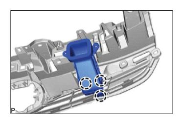
(b) Install the No. 3 air cleaner inlet with the 2 screws.
