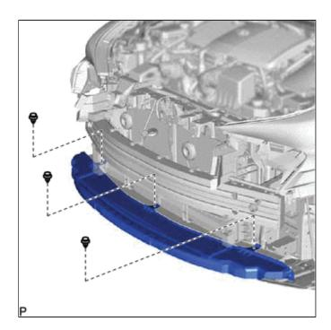
(a) Install the lower front bumper absorber with the 3 clips.
