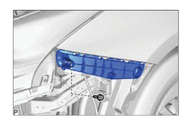
(b) Disengage the clip as shown in the illustration.
