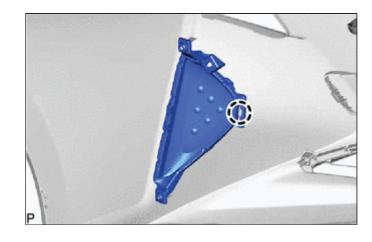
(b) Install the front bumper extension LH with the 2 screws.
