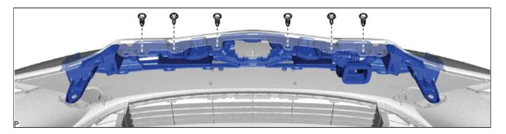
(b) Disengage the 15 claws as shown in the illustration to remove the radiator grille sub-assembly.
