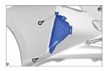
(b) Disengage the claw to remove the front bumper extension LH.
