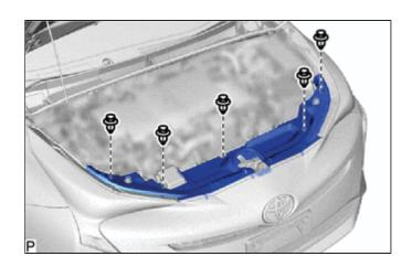
(b) Disengage the 2 guides and remove the radiator support opening cover as shown in the illustration.
