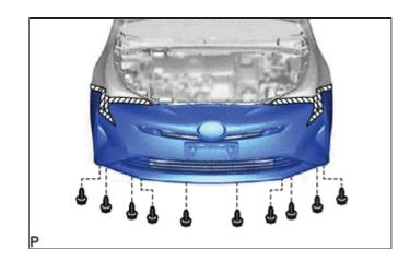
(e) Disengage the 4 claws as shown in the illustration.
