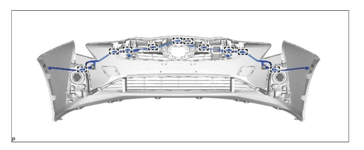
8. REMOVE MILLIMETER WAVE RADAR SENSOR ASSEMBLY (w/ Toyota Safety Sense P)
