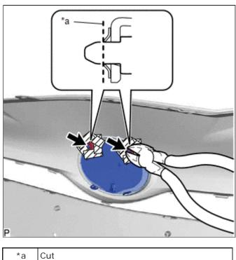
(3) Push the radiator grille emblem assembly to remove the 2 spring nuts as shown in the illustration.
