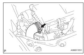
(b) Connect the No. 1 air cleaner inlet to the air cleaner case, and then tighten the clamp.
