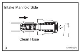
(3) Check that there no ventilation when air is applied to the intake manifold side. If there is ventilation, replace the ventilation valve.
