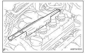
(b) Install the wire harness and brake master cylinder reservoir cover with the 3 bolts.
