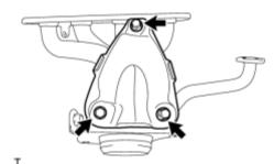
(a) Install the No. 2 exhaust manifold heat insulator with the 3 bolts.
