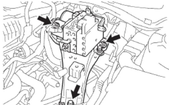
Removed actuator on bracket
