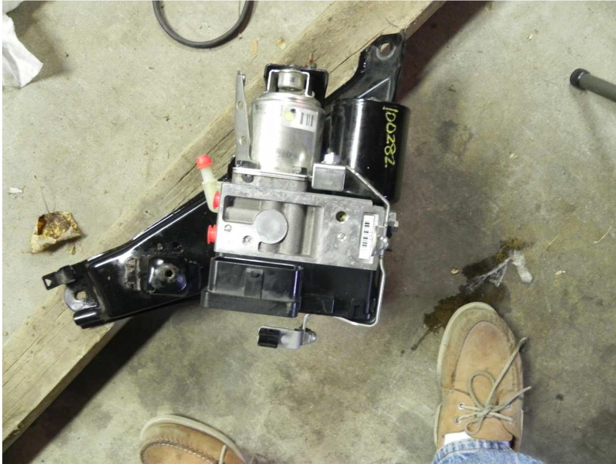
Remove damper from bracket, and remove bracket, replace actuator for reassembly.
