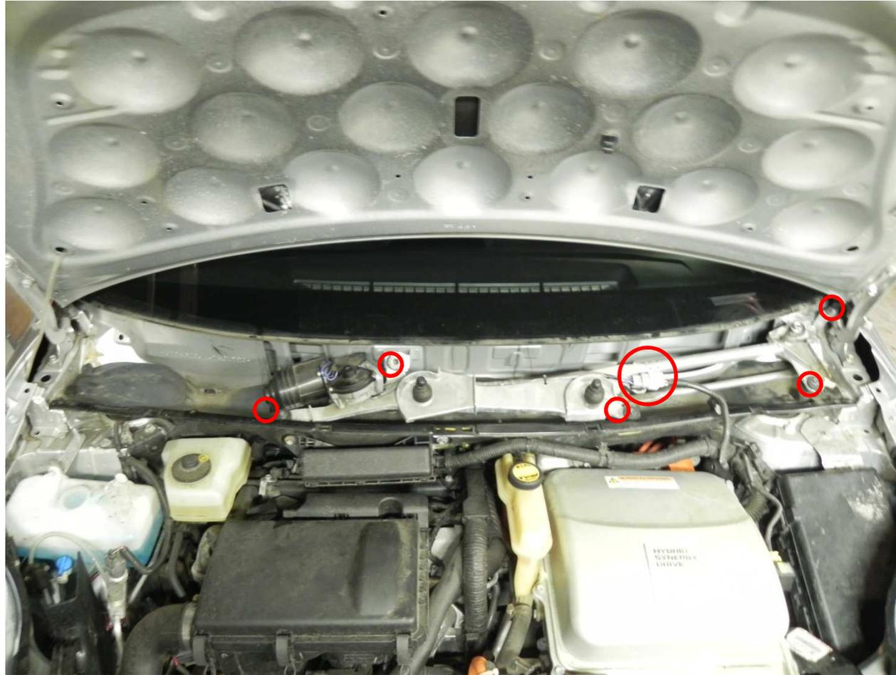
Remove cowling with 10mm socket
