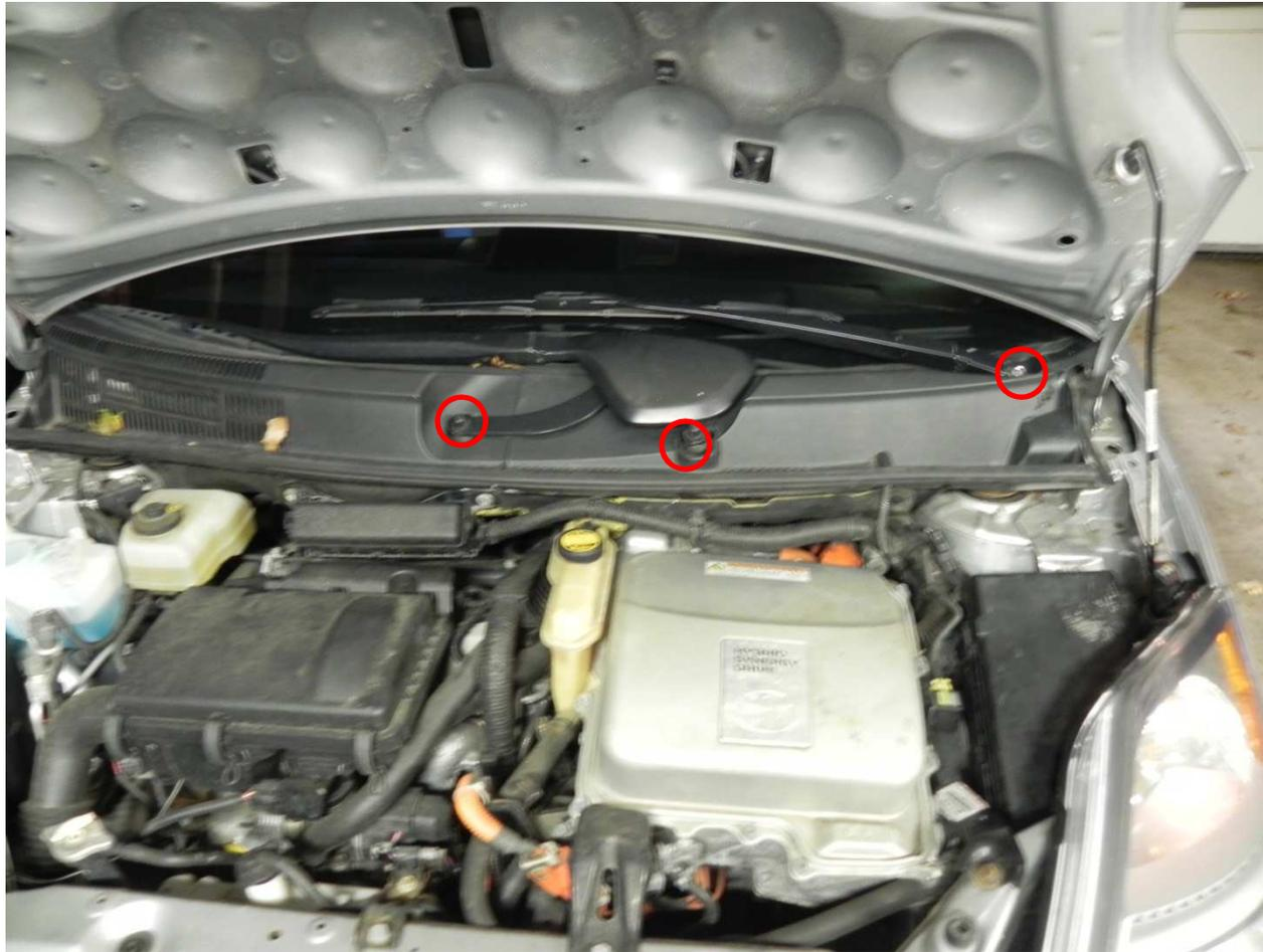
Remove Wiper motor with 10 mm socket and unplug connector
