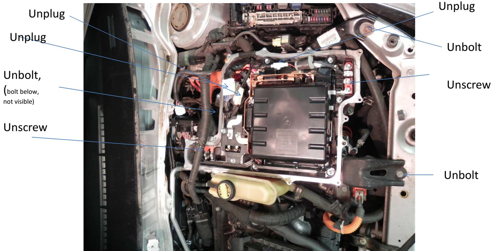
Lift up inverter, and place on left. I had to release two hose tie downs to move the inverter this far. It is not necessary to drain the fluid.
