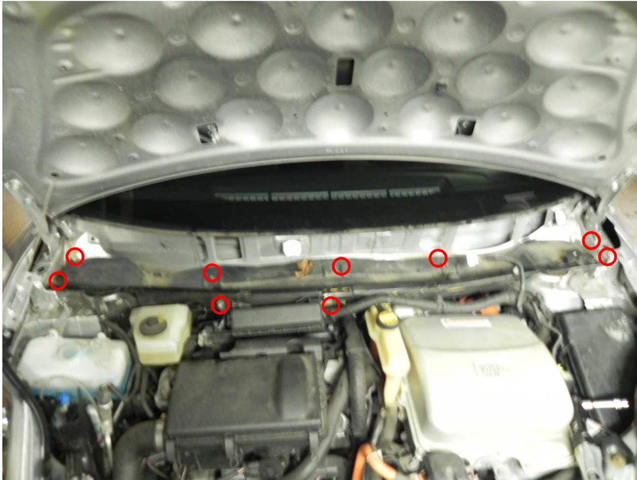
Top of Actuator is visible. Remove connector by pulling the white lock mechanism towards the front of the car. Then slide the cable side to the left. My connector was damaged by the accident, so the top par of the white mechanism is missing.
