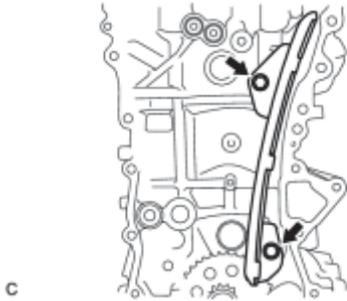
(a) Install the chain vibration damper with the 2 bolts.
