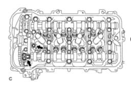
(a) Install 2 new gaskets to the camshaft bearing cap.
