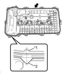
and the center of the cylinder head gasket tab is within 4 mm (0.157 in.).
