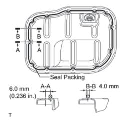
(b) Apply a continuous bead of seal packing (Diameter 4.0 mm (0.157 in.)) as shown in the illustration.
