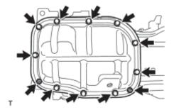
(c) Install the No. 2 oil pan with the 10 bolts and 2 nuts.
