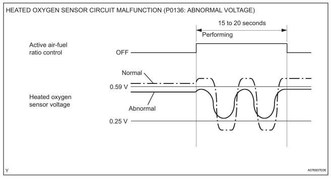
Oxygen Storage Capacity Detection in the Heated Oxygen Sensor Circuit (P0136, P0137 or P0138)
