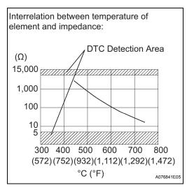
During normal feedback control of the air-fuel ratio, there are small variations in the exhaust gas oxygen concentration. In order to continuously monitor the slight variation of the signal from the oxygen sensor while the engine is running, the impedance\* of the sensor is measured by the ECM. The ECM detects that there is malfunction in the sensor when the measured impedance deviates from the standard range. \*: The effective resistance in an alternating current electrical circuit.
