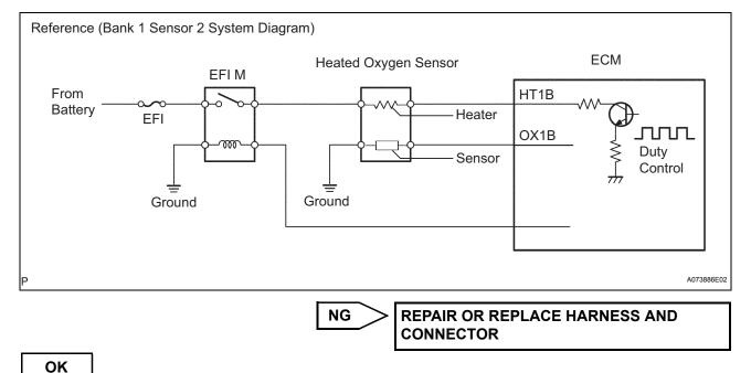
**REPLACE HEATED OXYGEN SENSOR**
