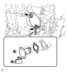
(b) Install a new gasket, the bracket and chain tensioner with the 2 nuts.
