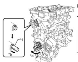
(d) Turn the crankshaft clockwise and check that the plunger is extended.
