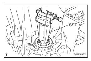
(b) Using SST, tap out the oil seal. **SST 09308-00010**
