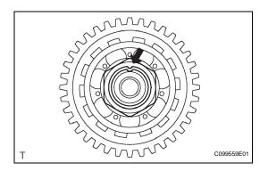
(c) Set the differential drive pinion in a vise and tighten a new nut using a deep socket wrench.
