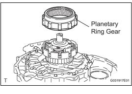
(9) Install the planetary ring gear.
