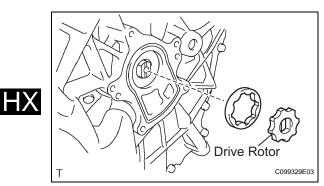
5. REMOVE TRANSAXLE OIL PUMP DRIVE ROTOR
