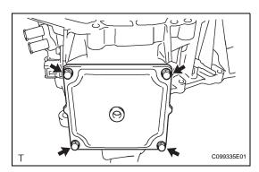
(b) Remove the 4 bolts and power cable cover.
