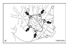
(b) Apply adhesive to the first 2 or 3 threads of the bolt end.
