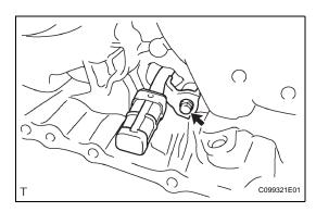
O-ring O-ring Transmission Oil Strainer
