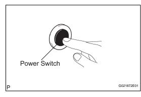
(b) Turn the power switch OFF when the vehicle is stopped.
