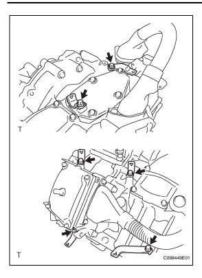
(b) Remove the 6 bolts shown in the illustration and clamp.
