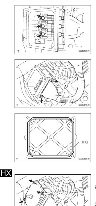
(c) Install the generator cable (terminals) with the 3 bolts.
