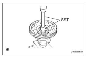
(g) Using a chisel, caulk the external circumference of the differential case straight pin hole.
