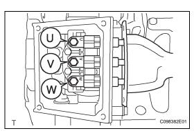
(2) Remove the 2 bolts from the generator cable.
