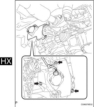
(b) Install the shift control actuator to the hybrid vehicle transaxle with the 3 bolts.
