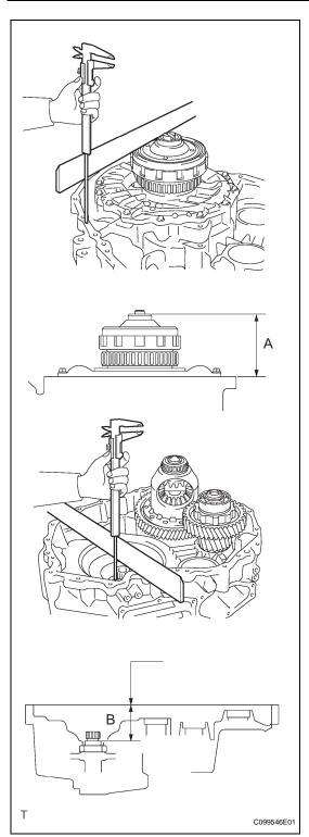
(11) Using a straightedge and vernier caliper, measure dimension A as shown in the illustration.
