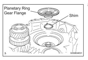
8. REMOVE PLANETARY RING GEAR FLANGE(a) Remove the planetary ring gear flange and shim.
