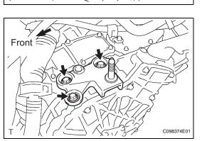
24. REMOVE NO. 3 ENGINE MOUNTING BRACKET(a) Remove the 3 bolts and engine mounting bracket.
