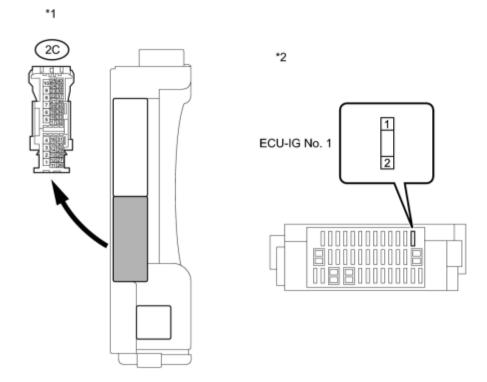
(b) Remove the ECU-IG No. 1 fuse from the driver side junction block assembly.
