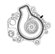
(a) Install a new water pump gasket.
