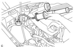
(b) Add engine coolant to the radiator and install the radiator cap tester.
