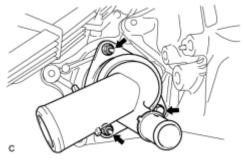
(b) Install the water inlet with thermostat sub-assembly with the 2 nuts and bolt.
