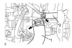
(c) Connect the No. 2 radiator hose and No. 3 water by-pass hose.
