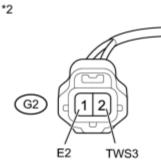
(b) Disconnect the No. 3 meter circuit plate connector.
