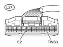
(a) Disconnect the engine coolant temperature sensor (for exhaust heat recirculation system) connector.
