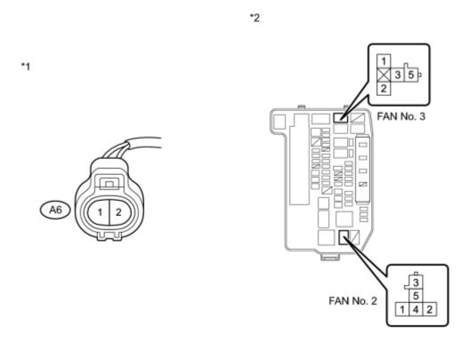
(b) Remove the FAN No. 2 relay and FAN No. 3 relay from the engine room relay block.
