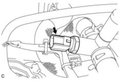
(a) Using a union nut wrench (19 mm), install the engine coolant temperature sensor.
