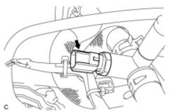
(b) Using a union nut wrench (19 mm), remove the engine coolant temperature sensor.
