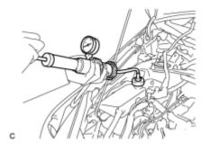
(b) Fill the radiator and reservoir with coolant, and then attach a radiator cap tester.
