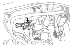
(b) Connect the engine coolant temperature sensor connector.
