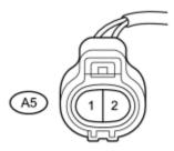
(b) Measure the resistance according to the value(s) in the table below.
