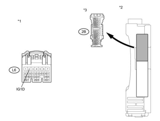
(b) Disconnect the power management control ECU connector.
