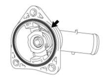
(a) Install a new gasket on the water inlet with thermostat sub-assembly.
