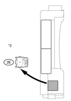
(a) Disconnect the driver side junction block assembly connector.
