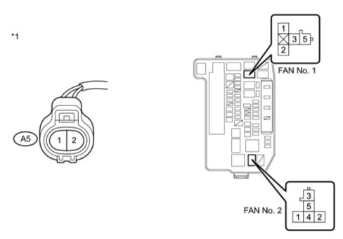
(b) Remove the FAN No. 1 relay and FAN No. 2 relay from the engine room relay block.
