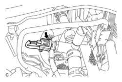
(a) Disconnect the engine coolant temperature sensor connector.
