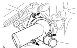
(b) Remove the 2 nuts, bolt and water inlet with thermostat sub-assembly.
