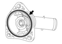
(c) Remove the gasket from the water inlet with thermostat sub-assembly.
