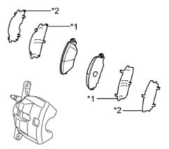
(a) Remove the front No. 1 anti-squeal shim and front No. 2 anti-squeal shim from each brake pad.
