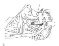
(a) Remove the front No. 2 disc brake cylinder slide pin from the front disc brake cylinder mounting.
