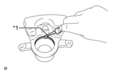
tape, remove the piston seal from the disc brake cylinder assembly.
