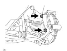
(a) Install the front disc brake cylinder mounting to the steering knuckle with the 2 bolts.
