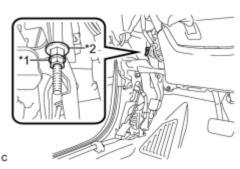
(b) Loosen the lock nut and adjusting nut to completely release the parking brake cable.
