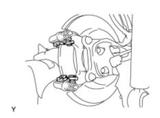
(a) Remove the 2 rear disc brake pad support plates from the disc brake cylinder mounting.
