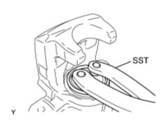
(a) Using SST, remove the rear disc brake piston by turning it counterclockwise.
