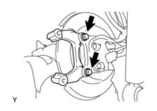
(a) Remove the 2 bolts and rear disc brake cylinder mounting from the axle beam.
