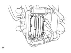
(a) Install the 2 rear disc brake pads to the rear disc brake cylinder mounting.
