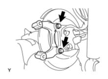
(a) Install the rear disc brake cylinder mounting to the axle beam with the 2 bolts.
