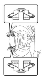
(a) Install the 2 rear disc brake pad support plates to the rear disc brake cylinder mounting.
