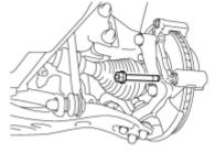
(b) Install the front No. 2 disc brake cylinder slide pin to the front disc brake cylinder mounting.
