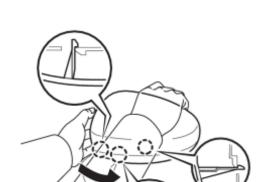
(b) Disengage the 3 claws and remove the outer mirror cover as shown in the illustration.
