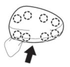
(a) Engage the 8 claws to install the outer mirror cover.
