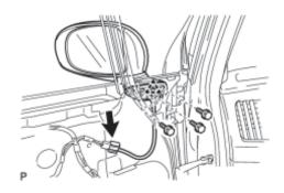
(a) Engage the clip to install the outer rear view mirror assembly.
