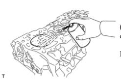
(a) Using a dye penetrant, check the intake ports, exhaust ports and cylinder surface for cracks.
