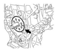
(a) Remove the crankshaft position sensor plate.
