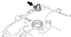
(a) Remove the bolt and camshaft position sensor.
