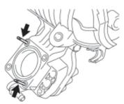
(a) Using an E6 "TORX" wrench, replace the 2 stud bolts.
