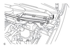
(2) Slide the hood to cowl top seal to engage the claw.
