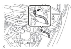
(1) Wait at least 2 minutes with the power switch off, and disconnect the reservoir level switch connector.
