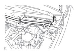
(1) Slide the hood to cowl top seal and disengage the claw.
