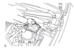
(2) Remove the brake master cylinder reservoir filler cap assembly.
