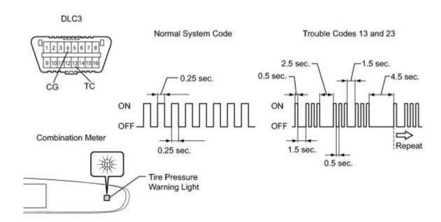
(b) Using SST, connect terminals 13 (TC) and 4 (CG) of the DLC3.
