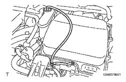
a. Loosen the bleeder plug shown in the illustration and connect a hose.
