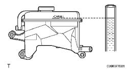
b. Add coolant until the level of coolant in the hose attached to the bleeder tank reaches the same level as the FULL line of the reserve tank.
