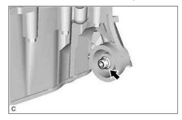
(a) Using a 12 mm hexagon socket wrench, install the oil filter union to the oil filter bracket.
