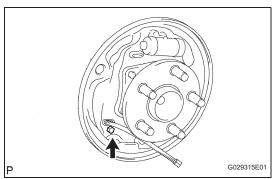
(c) Install the No. 3 parking brake cable to the backing plate with the bolt.
