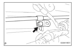
(e) Install the No. 1 parking brake cable to the floor with the clamp bolt.
