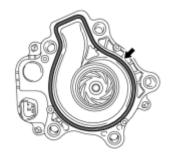
(a) Install a new water pump gasket.
