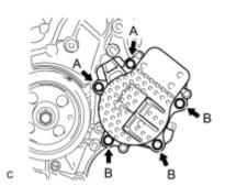
(b) Install the water pump assembly to the timing chain cover with the 5 bolts.
