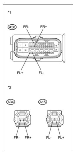
(a) Make sure that there is no looseness at the locking part and the connecting part of the connectors.
