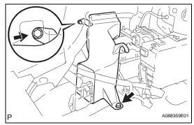
(d) Remove the bolt and screw, and then remove the guarter vent duct.
