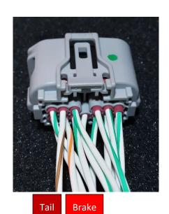
Must switch wires in CURT pins 5 & 12 with wires in pins 6 & 13, respectively, using terminal extraction tool:
