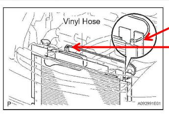
(d) Connect a vinyl hose to the bleeder plug of the radiator assembly and the radiator reservoir. HINT:
