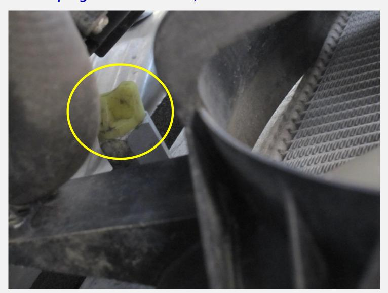
Connect Hose, Loosen the Drain Cock Plug of the Engine Block. Then Drain the Coolant into your pan. Patience AGAIN. Tighten the drain cock plug of the Engine Block. Then disconnect the hose.
