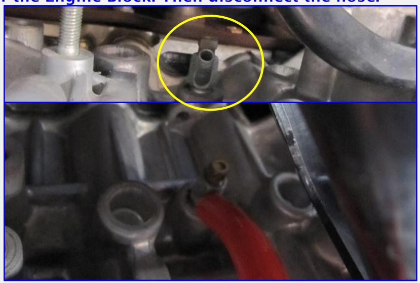
Connect Hose, Loosen the Drain Cock Plug of the Coolant Heat Storage Tank. Then Drain the Coolant into the pan. Tighten the drain cock plug of the Coolant Heat Storage Tank, then disconnect the hose.
