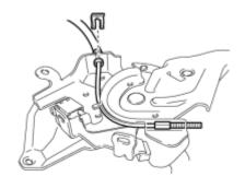
(c) Remove the clip from the No. 1 parking brake cable assembly.
