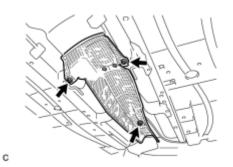
(a) Install the front No. 2 floor heat insulator with the 3 nuts.
