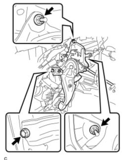
(a) Install the parking brake control pedal assembly with the bolt and 2 nuts
