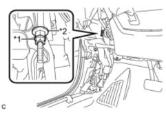
(c) Loosen the lock nut and the adjusting nut to completely release the parking brake cable.
