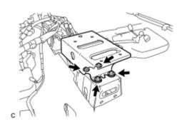
(a) Remove the 4 bolts and No. 2 belt anchor reinforcement sub-assembly.
