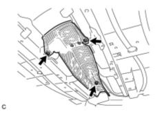
(a) Remove the 3 nuts and front No. 2 floor heat insulator.
