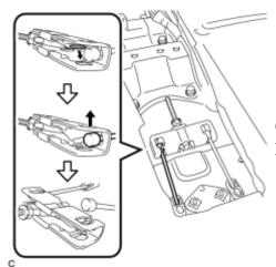
(a) Separate the No. 3 parking brake cable assembly from the No. 1 parking brake pull rod sub-assembly as shown in the illustration.
