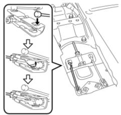
(b) Connect the No. 2 parking brake cable assembly to the No. 1 parking brake pull rod sub-assembly.
