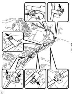
(a) Remove the 5 bolts and nut, and separate the No. 1 parking brake cable assembly.
