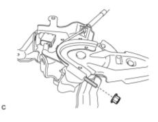
(a) Remove the adjusting nut.
