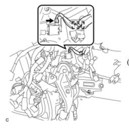
(b) Connect the parking brake switch connector.
