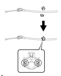
(a) Engage the 2 claws to install a new No. 2 parking brake cable clamp to the No. 3 parking brake cable assembly.
