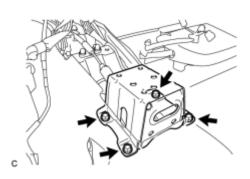
(a) Remove the 4 bolts and No. 3 belt anchor reinforcement sub-assembly.
