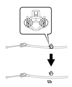
(a) Disengage the 2 claws to remove the No. 2 parking brake cable clamp from the No. 3 parking brake cable assembly.
