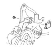
(a) Remove the screw and parking brake switch assembly from the parking brake control pedal assembly.
