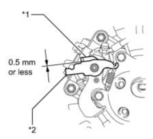
(a) Release the parking brake lever and check that the clearance measurement between the rear disc brake cylinder operation lever and the stopper is within the specified range.
