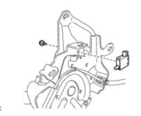
(a) Install the parking brake switch assembly to the parking brake control pedal assembly with the screw.
