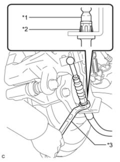
(c) Disconnect the No. 3 parking brake cable assembly from the rear disc brake cylinder assembly.
