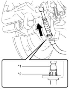
(b) Install the No. 3 parking brake cable assembly to the rear disc brake cylinder assembly.
