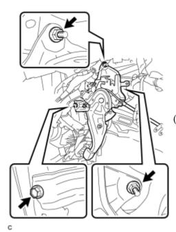
(e) Remove the bolt, 2 nuts and parking brake control pedal assem
