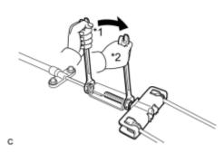
(a) Separate the No. 1 parking brake pull rod sub-assembly from the parking brake control pedal assembly as shown in the illustration.
