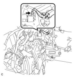
(c) Disconnect the parking brake switch connector.
