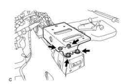
(a) Install the No. 2 belt anchor reinforcement sub-assembly with the 4 bolts.
