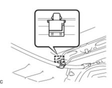
(d) Engage the clamp to install the No. 2 parking brake cable clamp.
