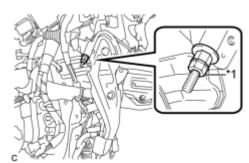
(f) Temporarily install the lock nut.
