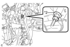
(a) Remove the lock nut and loosen the adjusting nut.
