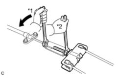
(a) Connect the No. 1 parking brake pull rod sub-assembly to the parking brake control pedal assembly as shown in the illustration.
