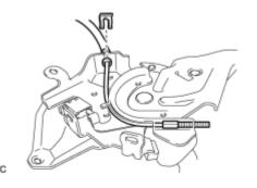
(b) Install the clip to the No. 1 parking brake cable assembly.
