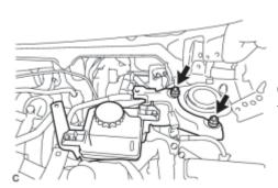
(a) Remove the 2 nuts and separate the brake master cylinder reservoir with bracket.
