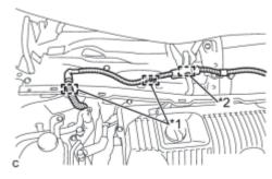
(a) Disengage the 2 clamps and guide of the wire harness.
