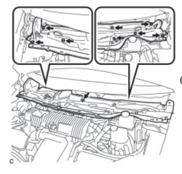
(d) Remove the 9 bolts and outer cowl top panel sub-assembly.
