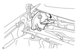
(b) Disengage the claw and bend the No. 1 heater air duct splash shield seal.
