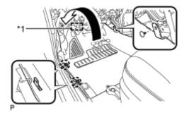
(c) Engage the fastener to install the floor carpet to the original position as shown in the illustration.
