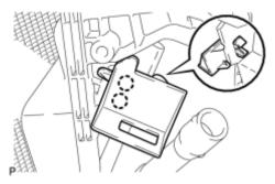
(a) Disengage the 2 claws and remove the console mounting bracket RH.
