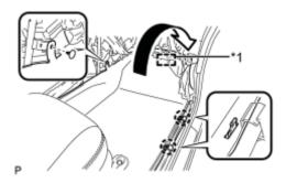
(c) Engage the fastener to install the floor carpet to the original position.
