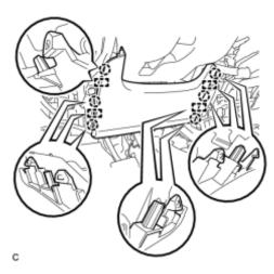
(e) Disengage the 6 claws and 4 guides to separate the driver side knee airbag assembly.
