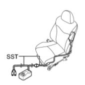
(1) Connect the SST connector to the front seat side airbag assembly connector.
