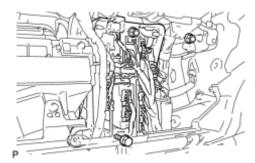
(b) Install the ECU integration box RH with the bolt and 2 nuts.
