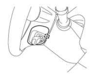
(a) Engage the claw to install the lower No. 2 steering wheel cover.
