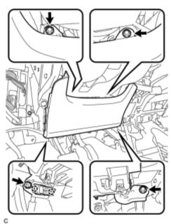
Confirm that the driver side knee airbag assembly is installed securely without any excessive gaps and is not protruding outward.
