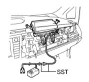
(1) Connect the SST connector to the instrument panel wire assembly.
