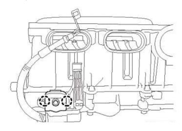
• Remove the nut from the No. 2 engine room wire.
