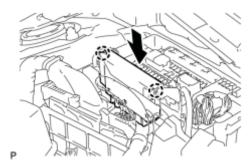
(b) Engage the 2 claws to install the integration relay as shown in the illustration.
