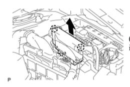
(a) Disengage the 2 claws and pull up the integration relay as shown in the illustration.
