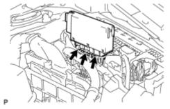
(b) Disconnect the 3 connectors and remove the integration relay.
