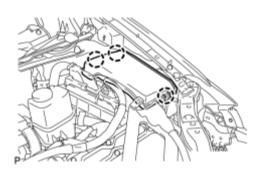
(a) Engage the 3 claws to install the No. 1 relay block cover.
