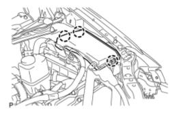
(a) Disengage the 3 claws and remove the No. 1 relay block cover.
