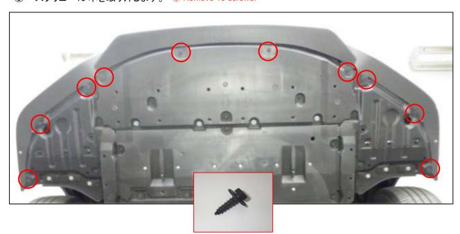
⑥ ツメのかん合3ヶ所を外します。(左右) ⑥ Remove the three mating points of the claws. (Left and right)
