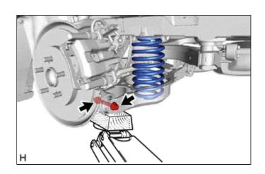
(e) Slowly lower the rear No. 2 suspension arm assembly, and then remove the rear coil spring.
