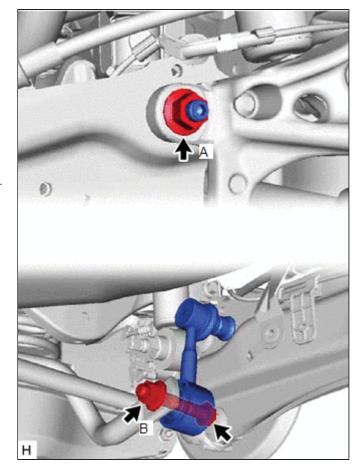
(b) Install the rear stabilizer link assembly LH with the bolt and nut (B).
