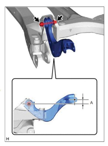
(b) Position the rear upper control arm assembly LH as shown in the illustration.
