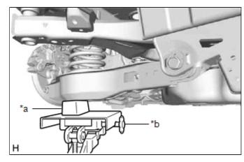
\*a Wooden Block (b) Remove the 2 bolts and separate the rear trailing arm assembly from the rear axle carrier sub-assembly.
