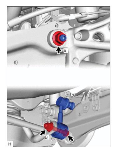
(b) Loosen the nut (B) of the rear stabilizer link assembly LH.
