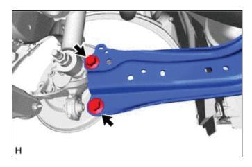
(c) Remove the 4 bolts and rear trailing arm assembly.
