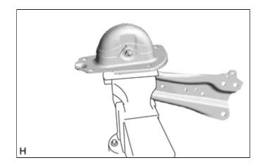
(b) Disengage the 4 claws and remove the rear suspension arm cover.
