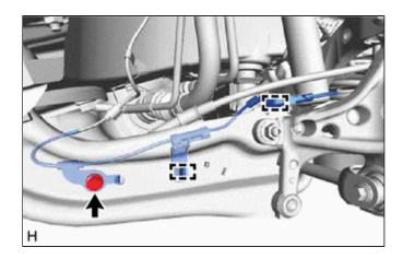
(b) Remove the bolt and separate the skid control sensor wire from the rear trailing arm assembly.
