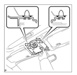
(a) Disengage the 4 clips and 2 guides as shown in the illustration.
