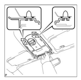
(a) Disengage the 4 clips and 2 guides as shown in the illustration.
