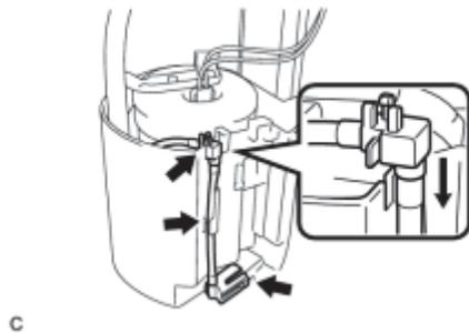
(f) Align the groove of the fuel pump filter hose with the cutout of the fuel sub-tank and install the hose.
