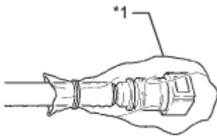
(6) Cover the disconnected pipe and connector with a plastic bag to prevent damage and contamination.
