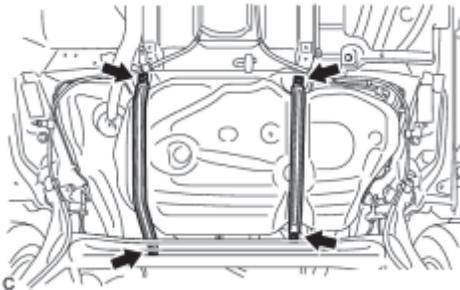
(c) Remove the 4 set bolts of the 2 fuel tank bands.
