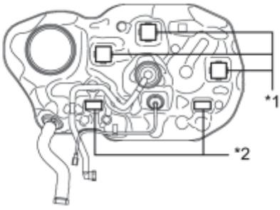
(a) Remove the 3 No. 1 fuel tank cushions and 2 No. 2 fuel tank cushions.
