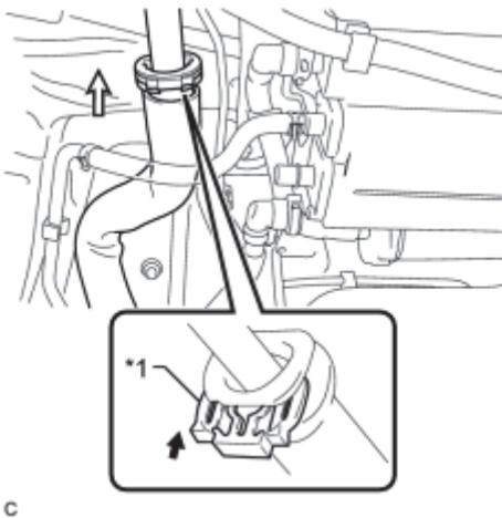
(a) Push in the hose connector to the filler pipe and install the retainer.
