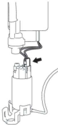
(b) Connect the fuel pump harness connector.
