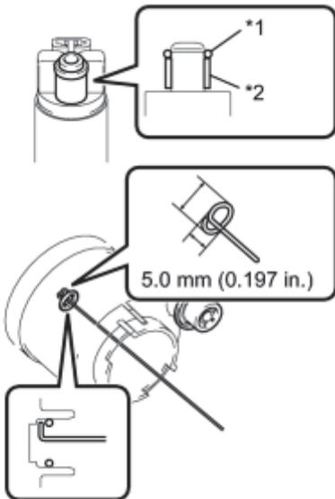
(g) Remove the O-ring and spacer from the fuel pump.
