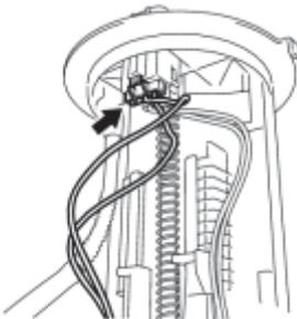
(c) Disconnect the connector of the fuel sender gauge assembly.
