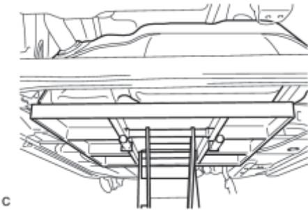
(b) Support the fuel tank using an engine lifter.
