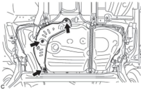
(a) Remove the 3 bolts and the No. 1 fuel tank protector.
