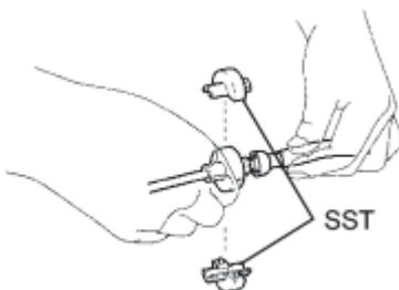
(4) Assemble SST to the connector as shown in the illustration.
