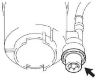
(a) Using a screwdriver with its tip wrapped in protective tape, remove the fuel pressure regulator assembly.
