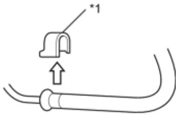
(2) Remove the No. 2 fuel pipe clamp.
