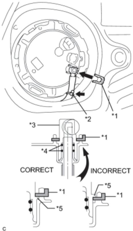
(a) Push the fuel tube joint in the plug of the fuel suction plate, then install the tube joint clip.
