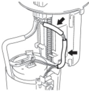
(b) Remove the 2 harness protectors from the wire harness.
