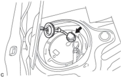
(b) Disconnect the fuel pump connector.
