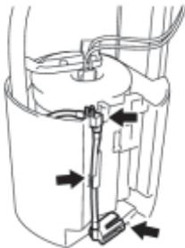
(b) Disconnect the fuel pump filter hose.
