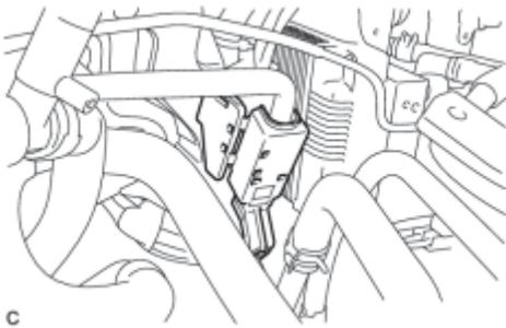
(5) Engage the lock claw and install the No. 1 fuel pipe clamp.
