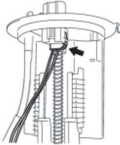
(a) Disconnect the connector of the fuel pump harness.
