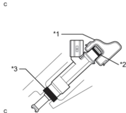
(b) Install the injector into the delivery pipe and cylinder head as shown in the illustration. Apply grease or gasoline to the contact surfaces of the injector before installing the injector.
