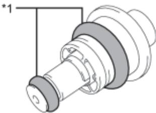
(b) Remove the 2 O-rings from the pressure regulator assembly.
