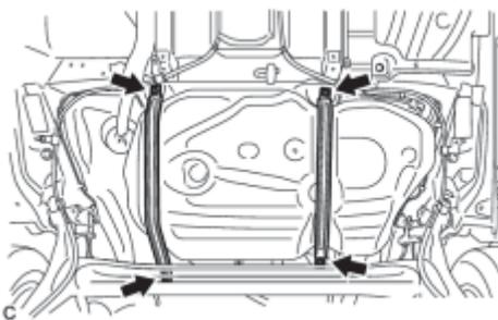
(c) Tighten the 4 set bolts of the 2 fuel tank bands.
