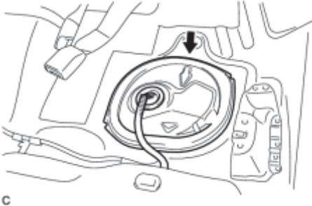
(a) Remove the rear floor service hole cover.
