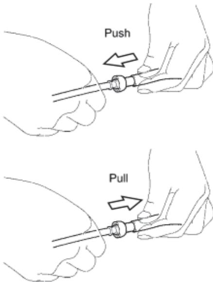
(2) Match the axis of the connector with the axis of the pipe, and push the pipe into the connector until the connector makes a "click" sound. If the pipe is difficult to push into the connector, apply a small amount of clean engine oil to the tip of the pipe.
