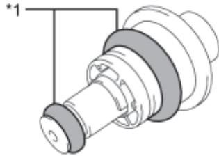
(a) Apply gasoline to 2 new O-rings and then install them to the fuel pressure regulator assembly.
