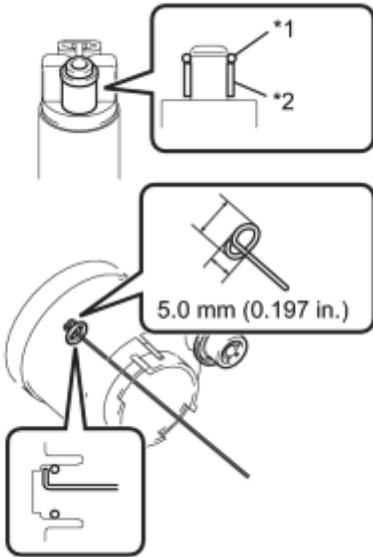
If the O-ring still remains in the fuel filter, remove it using a wire tip (1 mm diameter) that is formed as shown in the illustration.
