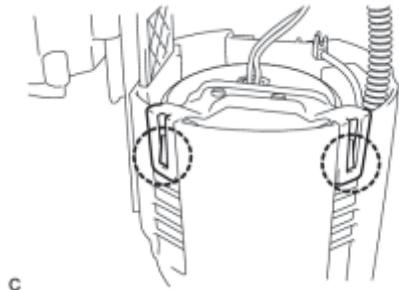
(e) Engage the 2 claws of the fuel suction support and install the fuel filter and the fuel pump onto the fuel sub-tank.
