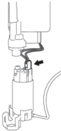
(f) Disconnect the fuel pump harness connector.
