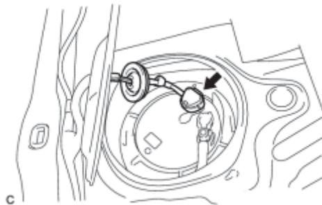
(b) Connect the fuel pump connector.
