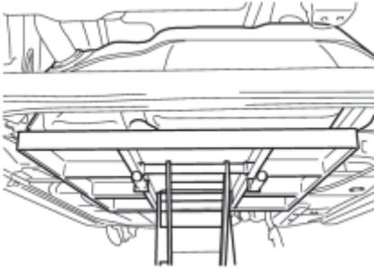
(b) Raise the engine lifter, then install the fuel tank to the vehicle.
