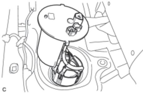
(a) Remove the fuel suction tube assembly with pump and gauge from the fuel tank.
