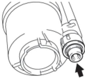
(b) Install the fuel pressure regulator assembly.
