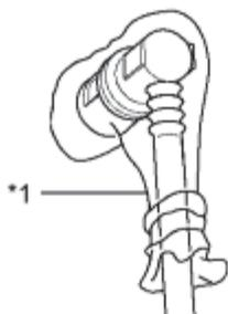
(4) Cover the disconnected pipe and connector with a plastic bag to prevent damage and contamination.
