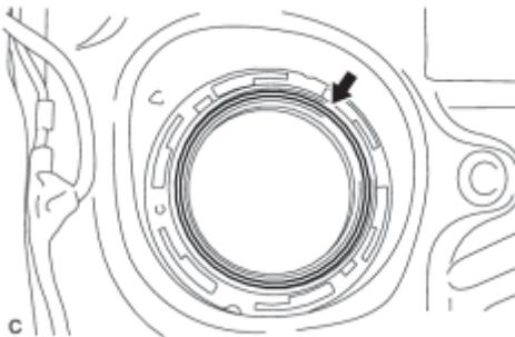
(b) Remove the gasket from the fuel tank.
