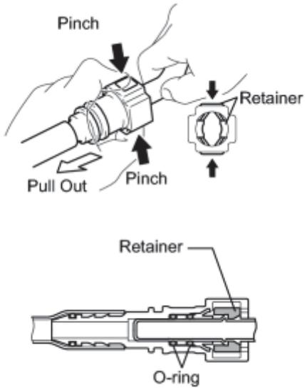
(5) Check that there is no dirt or other foreign objects on the contact surface of the disconnected pipe. Clean them away if necessary.
