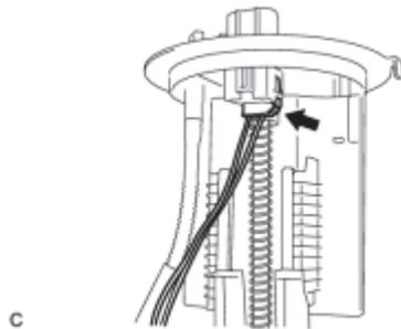
(g) Connect the connector of the fuel pump harness.
