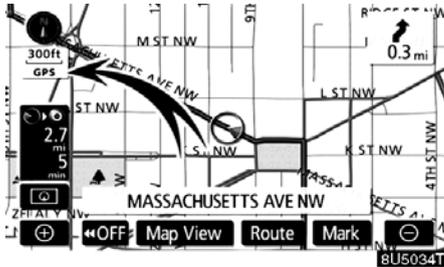
When your vehicle is receiving signals from the satellites, the “GPS” mark appears at the top left of the screen.
