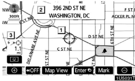
Use the scroll feature to move the desired point to the center of the screen for looking at a point on the map that is different from the current position of the vehicle.
