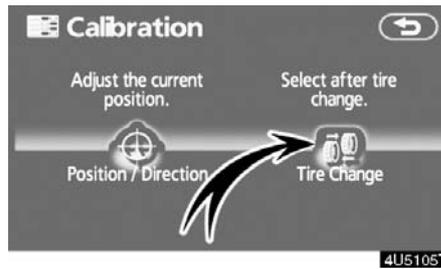
To perform a distance calibration procedure, touch "Tire Change" on the "Calibration" screen.
