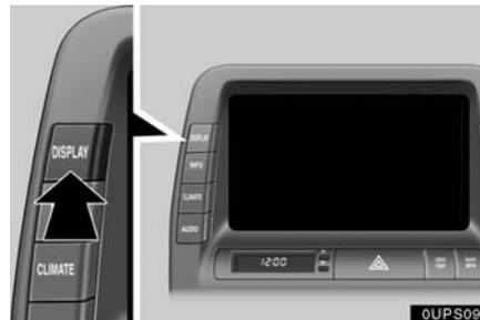
1. To display the “Display” screen, push the “DISPLAY” button.
