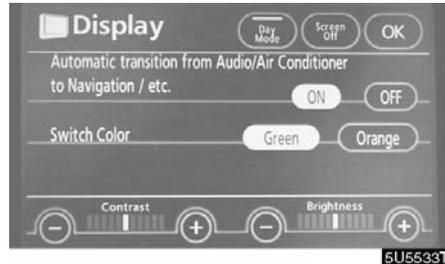
**2. Touch the desired button to adjust contrast and brightness.**
