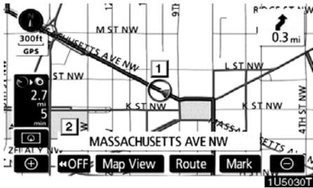
The current vehicle position mark (1) appears in the center or bottom center of the map screen.
