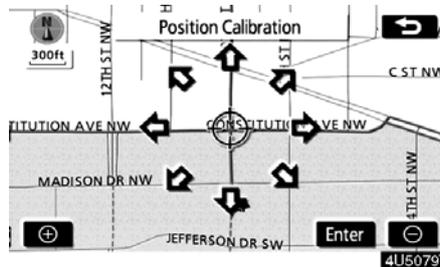
2. Touch the eight directional touch-screen button to move the cursor
