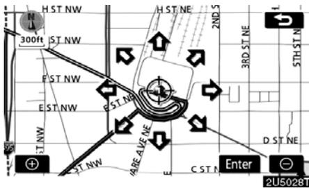
When an arrow facing the desired point is touched, the map scrolls in that direction. Releasing the finger from the arrow will stop the scrolling.
