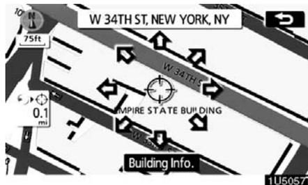
2. Using the eight-direction arrow, move the cursor to the position of the building to display building information.
