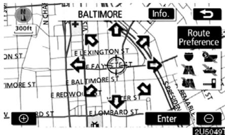
1. When an arrow facing the desired point is touched, the map scrolls in that direction.
