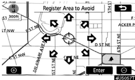
5. Touch the eight directional touch-screen button to move the cursor to the desired point on the map.
