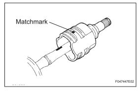
(h) Align the matchmarks and install the inboard joint onto the outboard joint.
