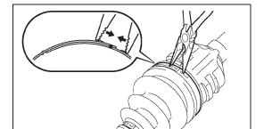
(b) When using a hook type:Using needle-nose pliers, unhook and remove the No. 2 inboard joint boot clamp.
