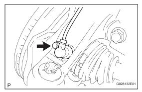
(b) Install the front speed sensor to the steering knuckle.
