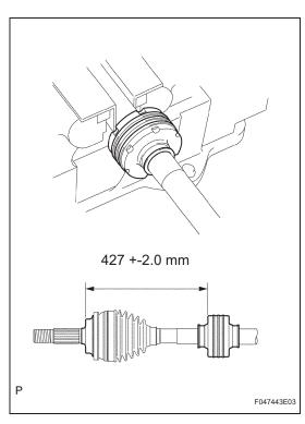
(a) Install the drive shaft damper to the outboard joint LH.
